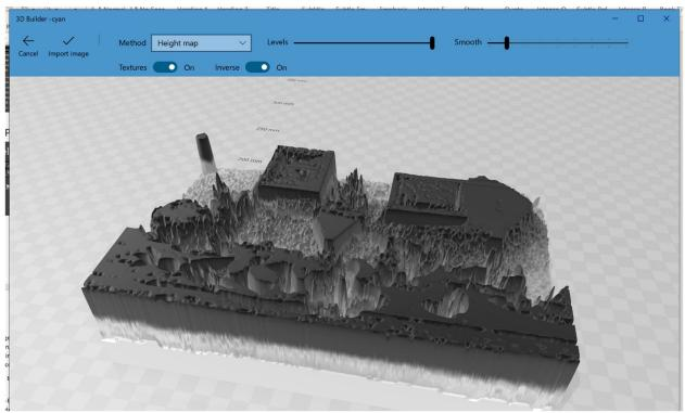
Notice the black dot makes the tallest level in the model and the white dot the lowest. Next step is to split the model so that the part below the white dot is cut away. For that click "Edit" and "split". This will show a green plane where the split is to occur.
